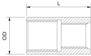
When it's necessary to splice rebars of different sizes, reduction coupler comes to help with it's top flexibility.
